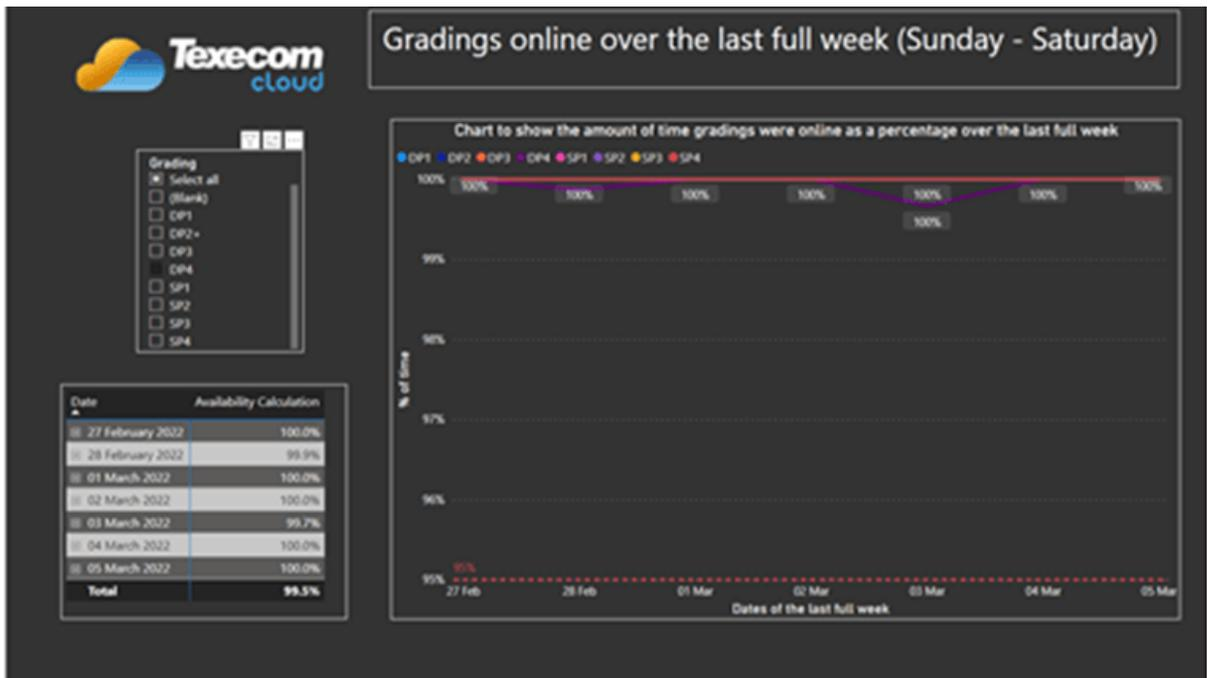
Texecom monitors each alarm system (panel/SmartCom) via polling and reporting times as defined by the category of the panels connection. In addition, the SmartCom monitors the network interface and identifies if the connection to the network switch has failed.
