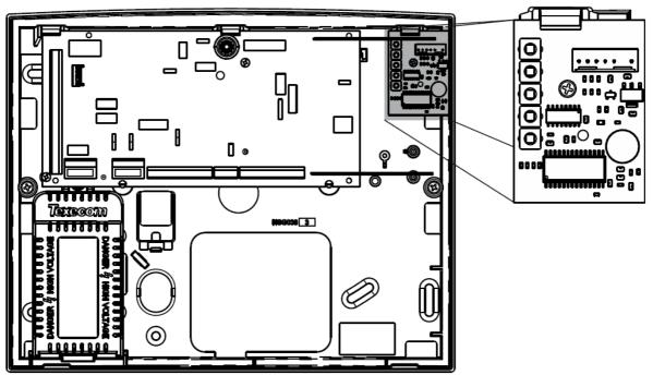
**Premier Elite** Large Polymer Housing (e.g. 24 & -W panels) mount to the inner wall of the housing
