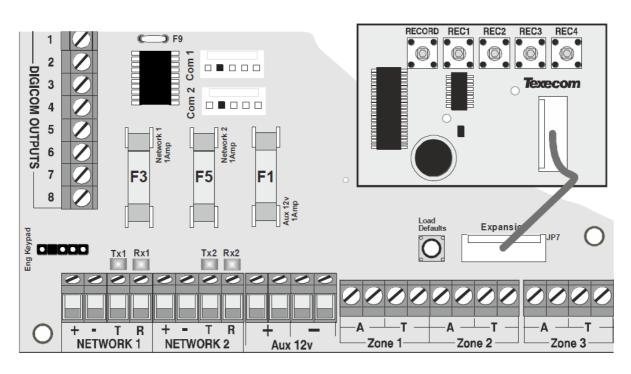
Figure 2 Premier Elite Speech Module Connected to Expansion Port on PCB
