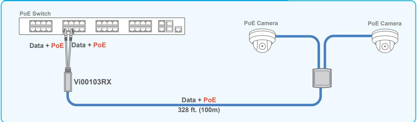
The NetMux™ Vi00103 can connect two cameras at standard UTP distances over a single cable.
