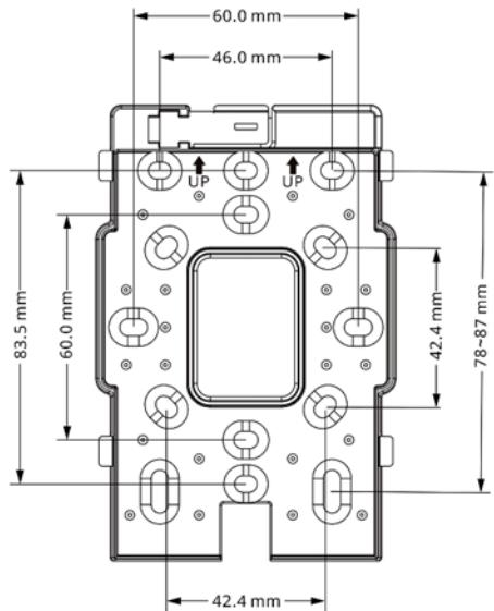
The access point can be installed on various junction boxes, including Chinese-standard and European-standard 86-mm junction boxes, American-standard 118-mm junction box, and South African-standard 120-mm junction box. To mount the access point on a Chinese-standard 86-mm junction box, follow these steps:
