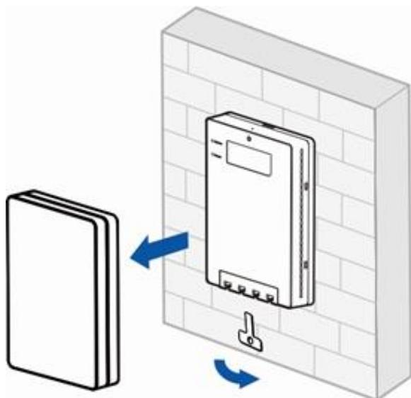
(2) Insert the T-key into the slot at the top of the device, and remove the device as indicated by the arrow.
