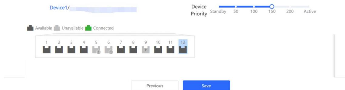
(7) Click **Next**. Use a 10GE cable to connect the VCS interfaces that you have selected. (The following figure shows an example of connecting Interface 12 of Device 1 to Interface 12 of Device 2.)
