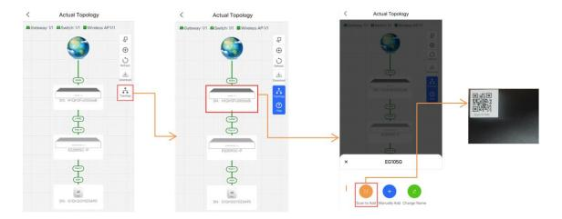
(3) After the device is detected, select its uplink port. And the device is added successfully.
