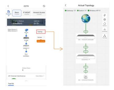
(2) Tap the **Topology** button, and select the existing managed device. To add an unmanaged downlink switch manually, select **Manually Add**.
