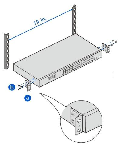
(2) Place the switch horizontally to an appropriate position in the rack. Use four M6 screws and matching cage nuts (both screws and nuts are to be provided by the user) to secure the other end of the mounting brackets to the square hole rack posts.
