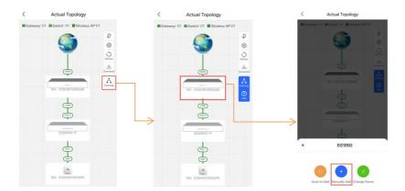
(3) Select the device model and its uplink port, and the device is added successfully.
