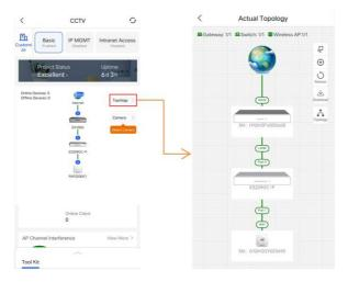
(2) Tap the **Topology** button, and select the existing managed device. To add an unmanaged downlink switch by scanning its QR-code, select **Scan to Add**.
