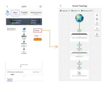
(2) Tap the **Topology** button, and select the existing managed device. To add an unmanaged downlink switch manually, select **Manually Add**.
