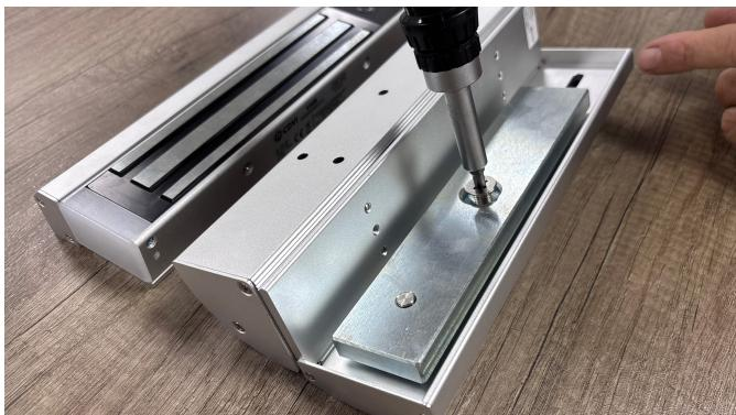
Install the armature plate assembly onto the Z-bracket as shown. Tighten the bolt (**E**) securely but ensure it still allows movement against the washer (**F**) for self-alignment. Otherwise, full holding force will not be achieved.
