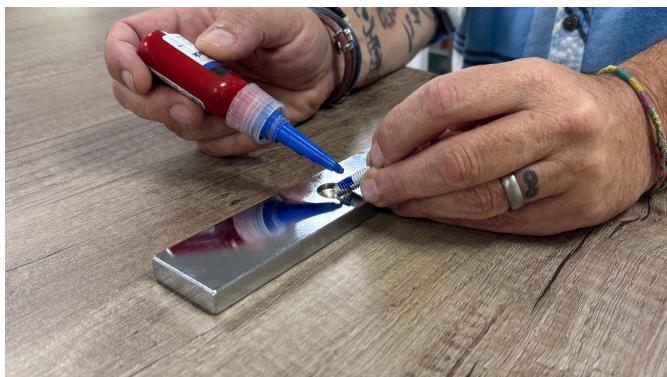
Once again, we highly recommend applying a Threadlock solution, such as Loctite, to the threads of the M8 bolt to prevent loosening during use.
