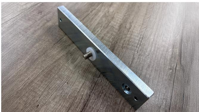
Insert the bolt (**E**) through the armature plate and fit the washer (**F**) on the opposite side as shown. The washer is essential to allow the armature to self-align with the magnet face.
