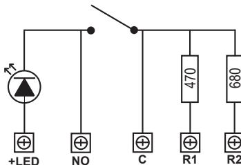
On the back of the call point there are 5 screw terminals connected to the internal PCB. Depending on where the wires are connected, the call point provides a series resistor, activates an internal LED or can simply provide a closing contact. If you choose to connect the +IN cable to the terminal marked +LED the call point, when operated, will switch on the internal red LED. Alternatively if you connect to the NO terminal the LED will not operate.
