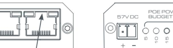
RJ45 Ethernet 10/100Base-Tx and POE connectors (auto speed, duplex, crossover, POE/POE Plus)
