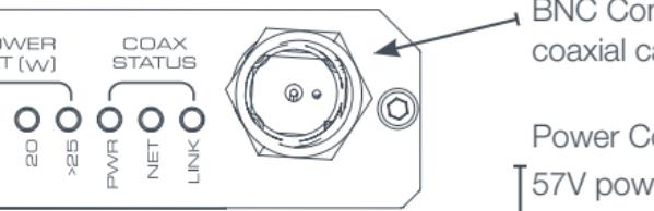
BNC Connector (for connection to any 75ohm coaxial cable)
