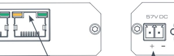
RJ45 Ethernet 10/100Base-Tx and POE connectors (auto speed, duplex, crossover, POE/POE Plus)
