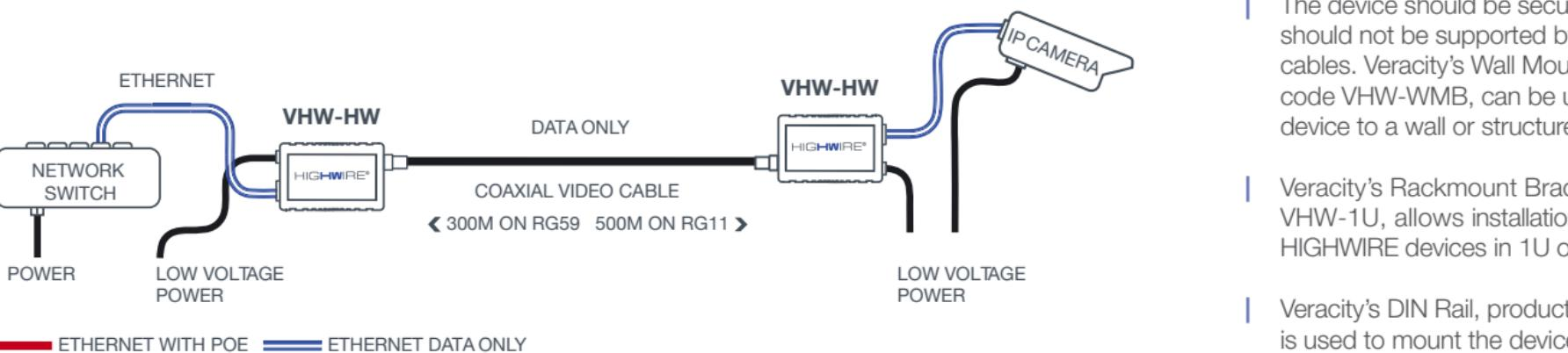
HIGHWIRE devices are used to convert conventional Ethernet to a signal that can be carried by 75ohm coaxial cables such as RG59, RG6 and RG11.
