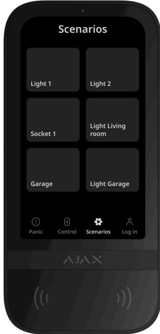
The separate keypad tab holds up to six buttons that control one automation device or a group of devices. Group scenarios provide more convenient control over multiple switches, relays, or sockets simultaneously.
