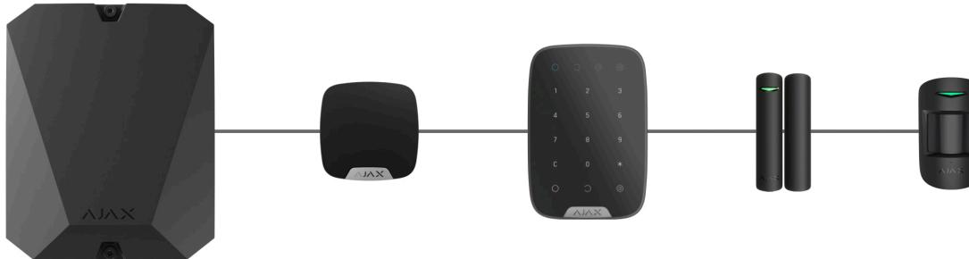
For the **Beam (Radial)** topology, be sure to install a 120 Ohm terminating resistor at the end of the line (included in the hub complete set). The terminating resistor is connected to the signal terminals of the last device on the line.
