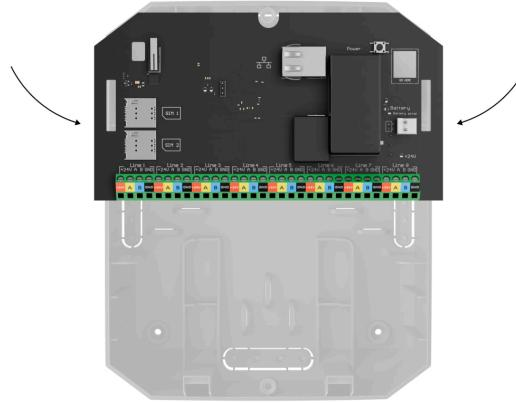
4. Connect the 12 V⎓ backup battery. Do not connect third-party power supplies. This could result in a failure of the control panel.
