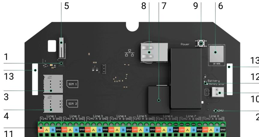
1. LED status indicator of the hub and connected communication channels.
