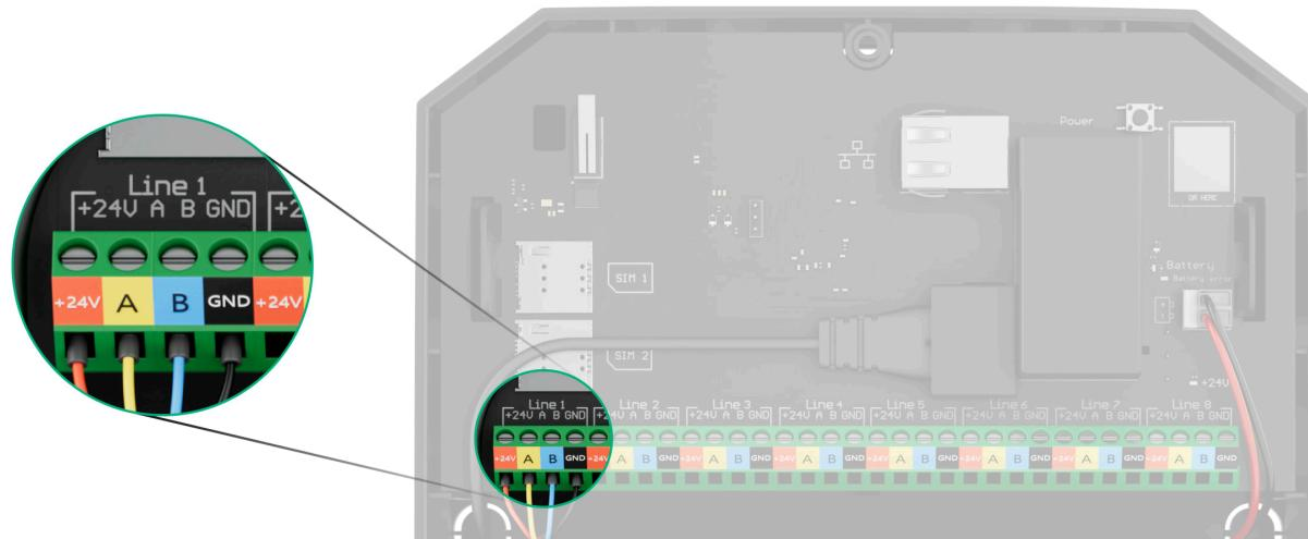
Superior Hub Hybrid has 8 Fibra lines. Numbers from 1 to 8 are indicated on the control panel board.
