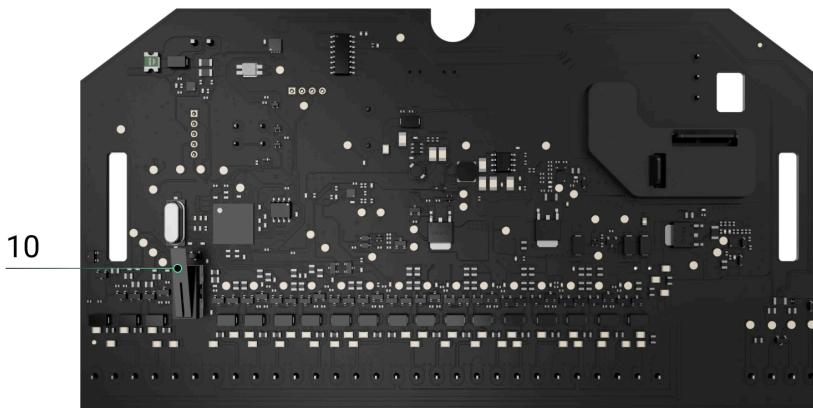
1. Fire detectors power supply terminals 10.5–15 V $\text{--}$ , up to 0.4 A.
