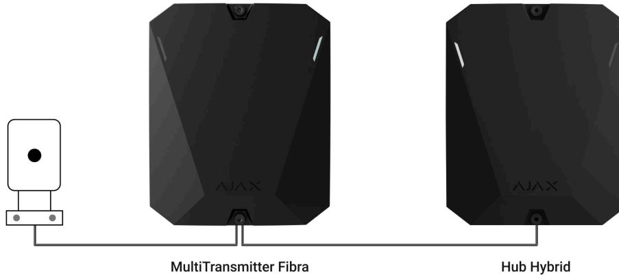
Superior MultiTransmitter Fibra is used to integrate alarm and auxiliary request alert buttons, indoor and outdoor motion detectors. As well as detectors that track opening, vibration, glass breaking, fire, gas and water leakage, etc.
