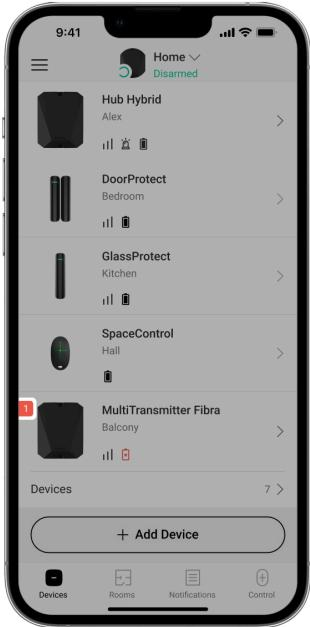
If a malfunction is detected in the integration module or a wired device connected to it, a malfunction counter will be displayed in Ajax apps in the upper left corner of the device icon.
