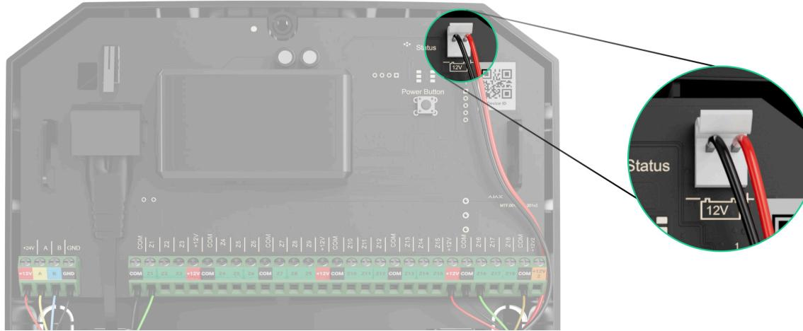
15. Connect the external 100-240 V~ power supply to the integration module.
