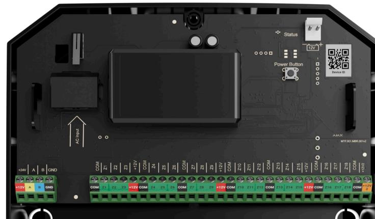
**Terminals for connecting Superior MultiTransmitter Fibra to the hub:**
