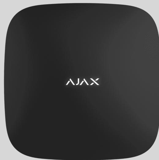
**Hub (2G) / (4G) Jeweller** is a control panel of the Ajax system. It controls the operation of connected devices and interacts with users, PROs, and security companies.
