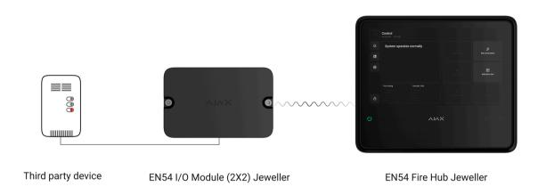
The module is powered by pre-installed batteries and does not require an external power supply. EN54 I/O Module (2X2) Jeweller monitors its operational state and informs the system of faults if any occur.
