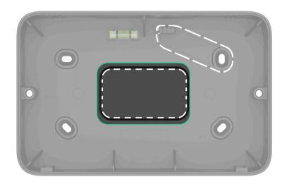
**To route the cable from the side, top, or bottom**, you can drill holes following the recesses on the module casing, considering the size of cable glands. There are two recesses on each side of the module. We recommend using a hole saw for plastic up to Ø20 mm.
