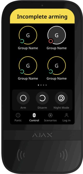
Superior KeyPad TouchScreen Fibra can participate in two-stage arming but cannot be used as a second-stage device. The two-stage arming process using Tag, Pass or smartphone is similar to using a personal or general code on the keypad.
