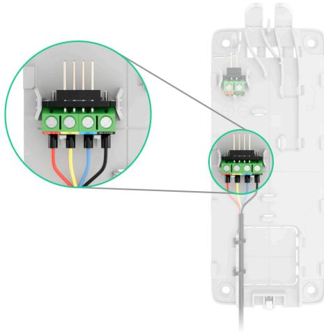
1. If Superior KeyPad TouchScreen Fibra is not the last device on the Fibra line, prepare a second cable in advance. Connect the wires to the keypad terminals according to the figure below. The ends of the wires of the first and second cables, which will be inserted into the detector terminals, must be tinned and soldered together, or crimped with a sleeve.
