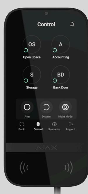
**Superior KeyPad TouchScreen Fibra** is a wired keypad with a touch screen designed for managing the Ajax system. Users can authenticate using smartphones, Tag key fobs, Pass cards, and codes. The device is intended for indoor use.
