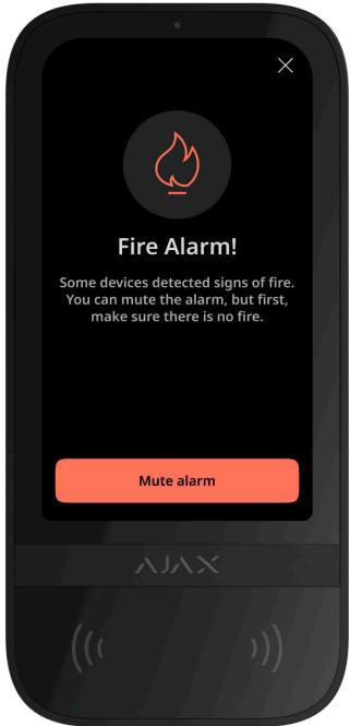
In case of a fire alarm in the system, users can mute it using Superior KeyPad TouchScreen Fibra.
