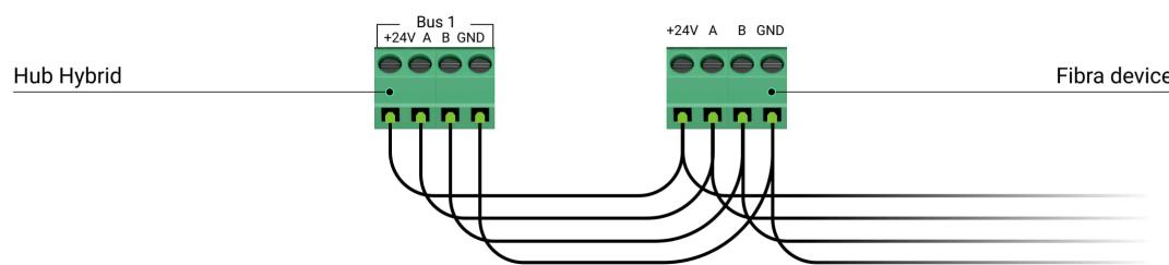
2. If Superior KeyPad TouchScreen Fibra is the last device on the line and you are using the **Beam (Radial) connection**, install a terminating resistor on
