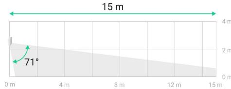
Vertical characteristics of the motion detection area
