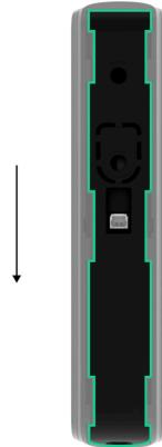
2. Fix the SmartBracket panel using double-sided tape or other temporary fasteners.
