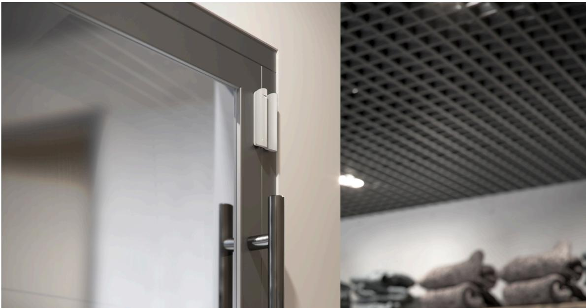
The detector must be placed on a moving part for Superior DoorProtect Plus Jeweller to detect shock and tilt.
