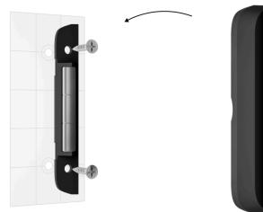
**9.** Tighten the holding screw on the bottom of the detector's and magnet's enclosure. The screw is needed for more reliable fastening and protection of the detector and the magnet from quick dismantling.
