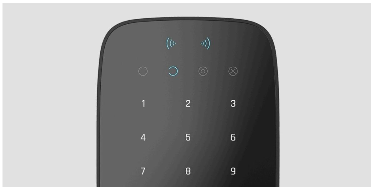
Superior KeyPad Plus Jeweller can be used in low-light conditions as it has a backlight. Pressing the buttons is accompanied by a sound signal. The backlight brightness and keypad volume are adjustable in the settings. If the keypad is not touched for 4 seconds, Superior KeyPad Plus Jeweller reduces the backlight brightness. After 8 seconds of inactivity, it enters power-saving mode and turns off the display.
