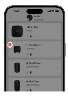
When a malfunction is detected, the Ajax app displays a malfunction counter on the device icon. All malfunctions are shown in the siren states. Fields with malfunctions will be highlighted in red.
