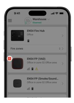
When an EN54 FireProtect (VAD) Jeweller fault is detected, an Ajax app displays a fault counter on the device icon. All faults are indicated in the device states. Fields with faults are highlighted in yellow. Also, faults are displayed in the **Control** tab of the CIE display. More details about the fault can be found in the **Event center** or **Fire zones** tabs of the CIE.
