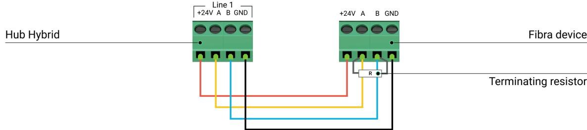
Line branching and the **Tree** topology are only allowed when using Superior LineSplit Fibra.
