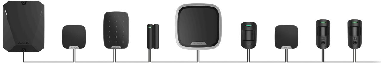
**Ring connection method** occupies two line outputs of the hub. If the ring breaks in one place, no device will be disabled. The ring reconfigures into two lines, which continue to operate normally. Users and security companies will receive notification of a break.
