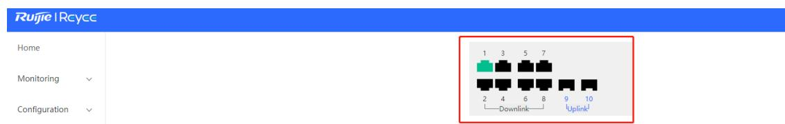
Different colors and shapes of the port icons represent different port statuses. See [Table 3-1](#) for details. Move the cursor over a port icon and the port status will be displayed, including the connection status, port rate, duplex mode, and flow control status.
