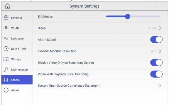
Figure 4-15 Enable Video Wall Playback Local Decoding
