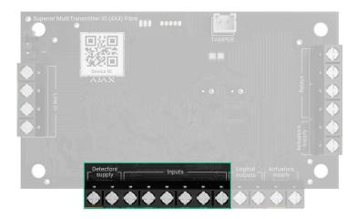
• **Z1-Z4** — inputs for connecting wired devices.
