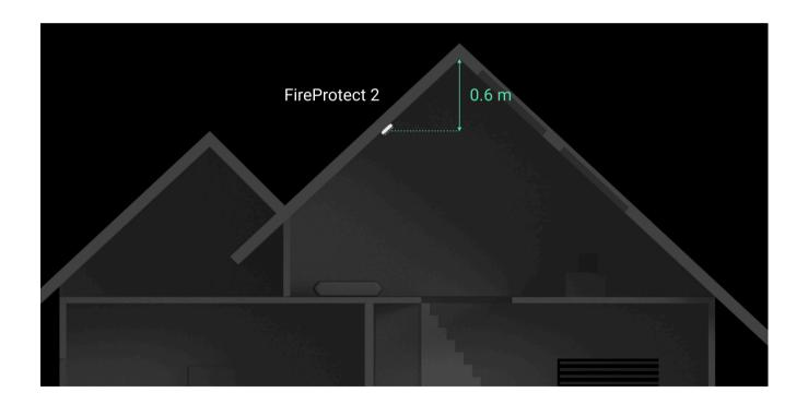
We do not recommend mounting the detector on a wall. This installation is acceptable if closely spaced beams or other obstacles interfere with the
