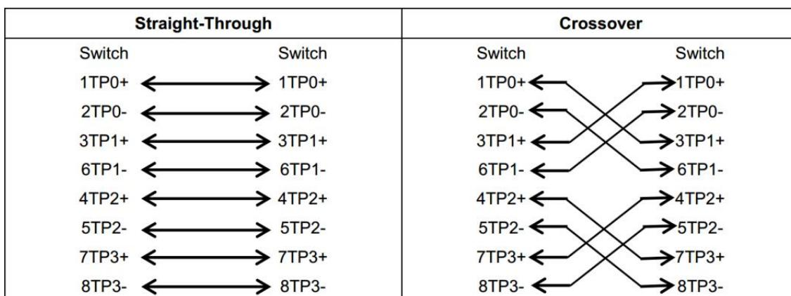
100BASE-TX/10BASE-T can be interconnected using cables of the preceding specifications. For 10 Mbps, the 100BASE-TX/10BASE-T port can be connected using 100-ohm Category 3, Category 4, and Category 5 cables; for 100 Mbps, the 100BASE-TX/10BASE-T port can be connected using 100-ohm Category 5 cables with a maximum connection distance of 100 meters. The following table shows 100BASE-TX/10BASE-T pin assignments.
