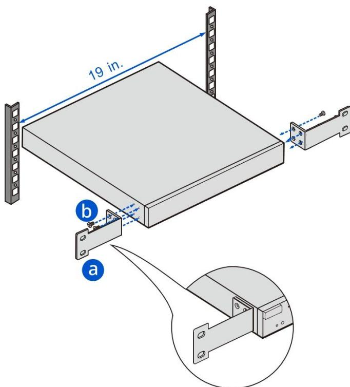
Follow the steps below to mount the switch in a 19-inch rack:
