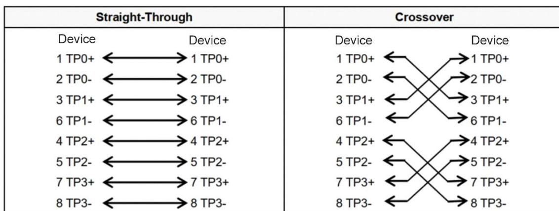
In addition to the above cables, the 100BASE-TX/10BASE-T can also use 100-ohm Category-3, 4, 5 cables for 10 Mbps, and 100-ohm Category-5 cables for 100 Mbps, both of which can be up to 100 m. [Table 6-1](#) shows the pinouts of the 100BASE-TX/10BASE-T.
