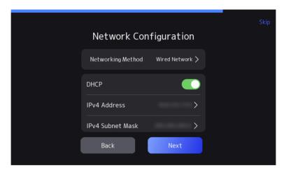
**Figure 2-4 Wired Network Configuration**
