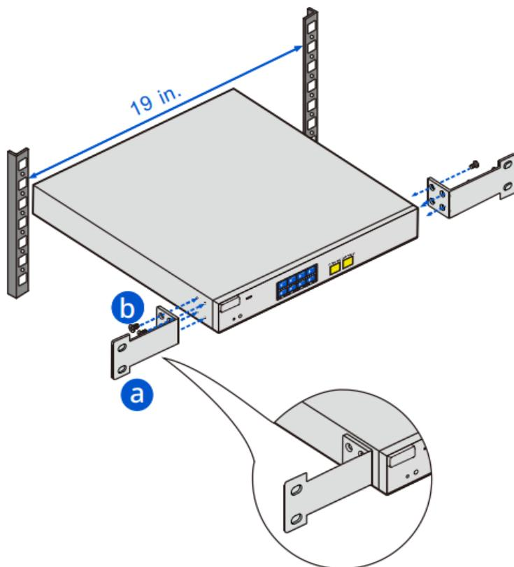
Step 2: Use the supplied M6 screws and cage nuts to securely attach the mounting brackets to the rack.
