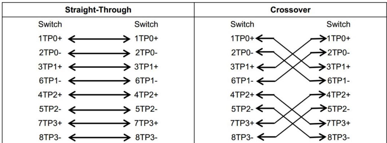
In addition to the preceding cables, the 100BASE-TX/10BASE-T can also use 100-ohm Category-3, Category-4, and Category-5 cables for 10 Mbps, and 100-ohm Category-5 cables for 100 Mbps, both of which can be up to 100 m. Figure A-2 shows the pinouts of the 100BASE-TX/10BASE-T.
