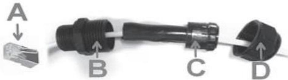
(4) Insert the crystal connector of the network cable into the ETH/PoE port on the AP and tighten the cable gland for B (split gasket), C (grommet), and D (compression cap) in sequence.
