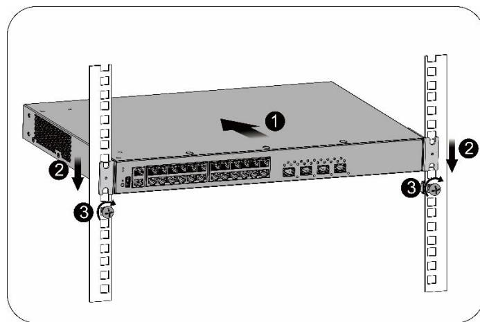
(4) Insert screws into the other two cage nuts and tighten them.
