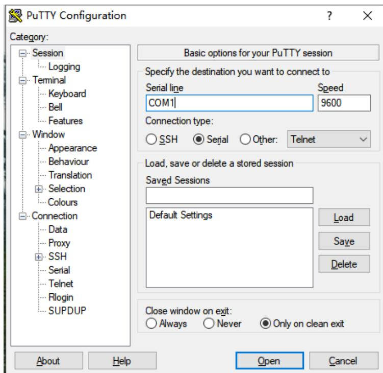
(3) Select **Serial**. The serial port parameter setting page is displayed. Set **Speed** to **9600**, **Data bits** to 8, **Stop bits** to 1, **Parity** to **None**, and **Flow control** to **None**.
