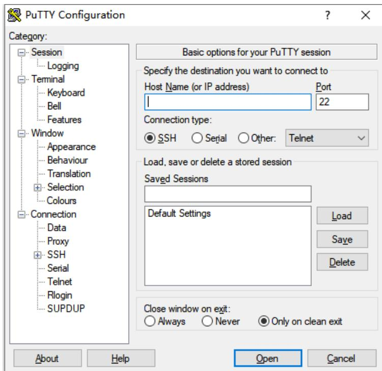
(2) Select **Serial**, and enter the serial port in **Serial line** and baud rate in **Speed**.
