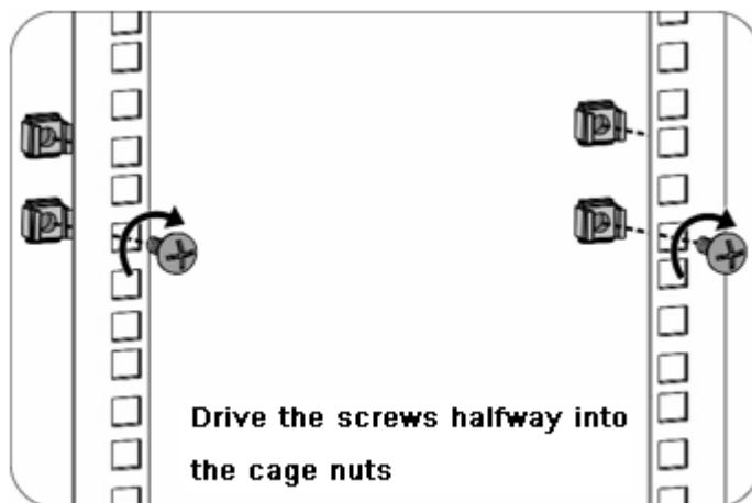
(3) Secure the switch on the rack rails by tightening the screws.
