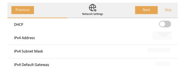
**Figure 2-3 Network Parameters**
