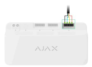
**7.** Connect the wires to the LineSupply output terminals according to the diagram below. Ensure the correct polarity and order of the wire connections. Secure the cable firmly to the terminals.
