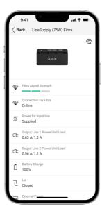
The states include information about the device and its operating parameters. You can find the states of LineSupply in the Ajax app:
