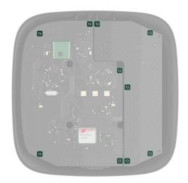
**6.** Carefully remove both boards, keeping them in the same plane and not disconnecting them. There is a connector between boards: do not break it.
