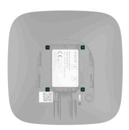
**5.** Remove the screws attaching the boards to the device body.
