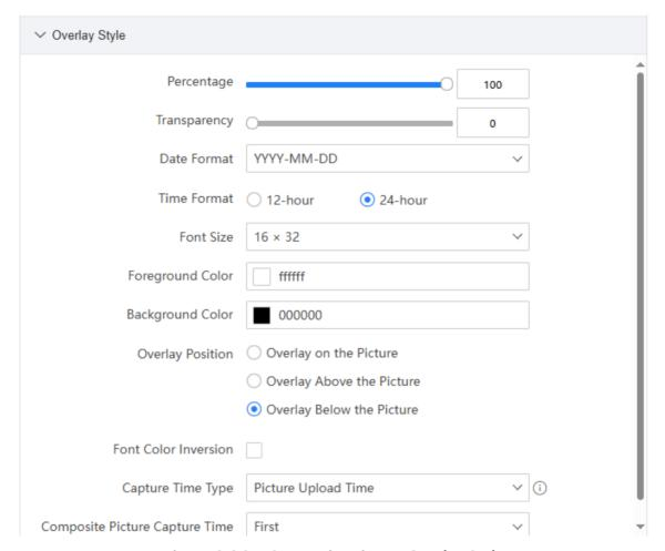
Figure 6-6 Set Composite Picture Overlay Style
