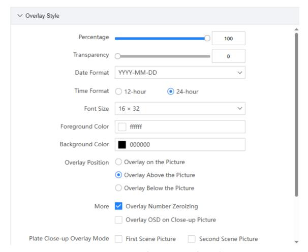
Figure 6-4 Set Single Picture Overlay Style
