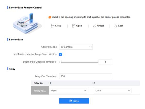
Figure 5-2 Control Barrier Gate
