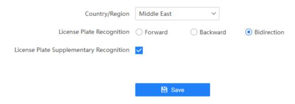
Figure 6-1 Set License Plate Recognition Parameters
