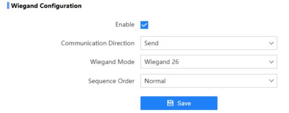
**Figure 5-5 Set Wiegand Parameters**
