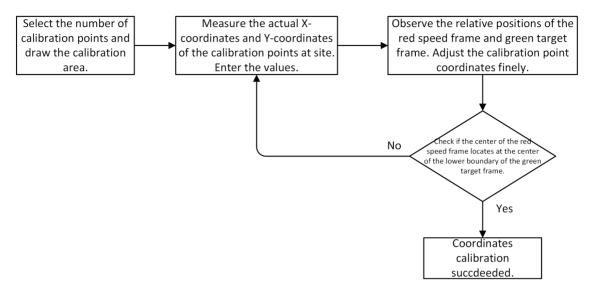
Figure 7-3 Manual Calibration Flow
