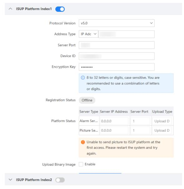
Figure 3-12 Connect to ISUP Platform
