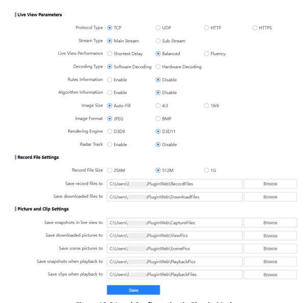
Figure 10-2 Local Configuration in Plug-in Mode
