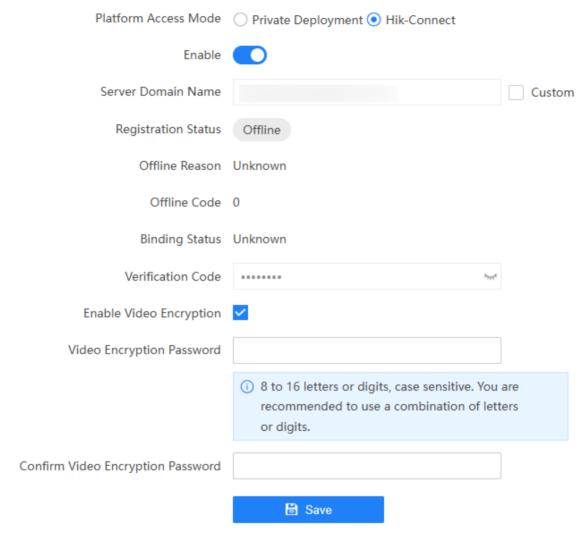
Figure 3-14 Connect to Hik-Connect (V2.0)
