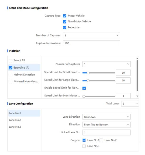
**Figure 4-1 Set Smart Monitoring Capture**
