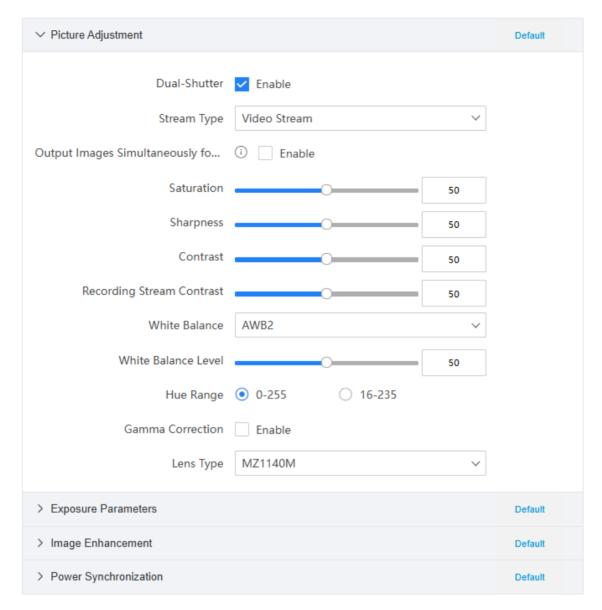
**Figure 12-1 Set Camera Parameters**
