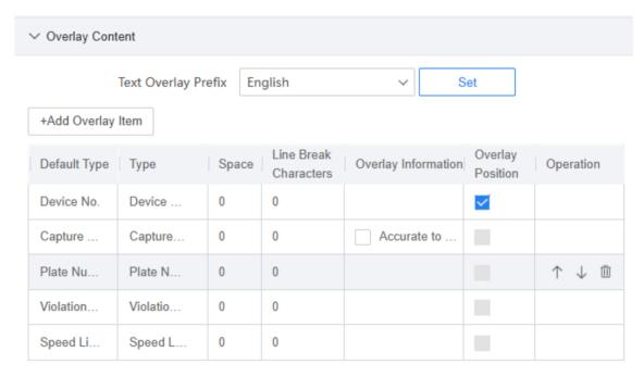
**Figure 6-5 Set Single Picture Overlay Content**
