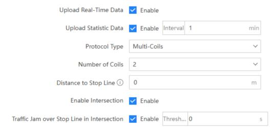
**Figure 4-7 Set Traffic Flow Detection**
