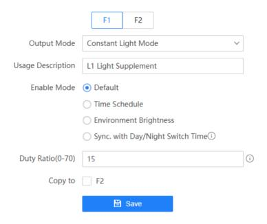
**Figure 6-2 Set Supplement Light Parameters**
