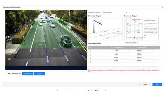
**Figure 7-4 Manual Calibration**
