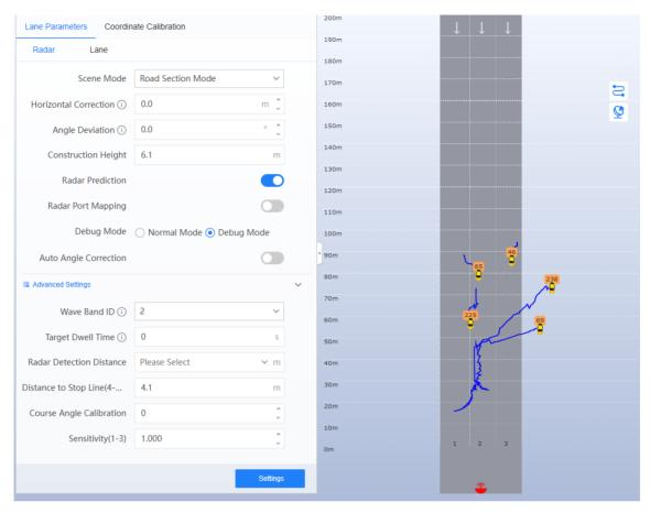
**Figure 7-1 Set Radar Parameters**
