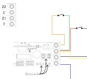
Remove the jumper to enable the external tamper terminal.
