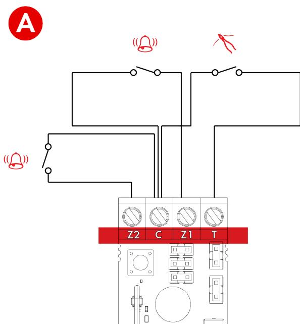
The device has four terminals that can be wired to utilise external inputs. The inputs must be wired in a double pole configuration between the common (C) and the zone/tamper terminal.
