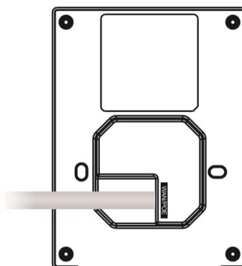
(3) Align the screw holes on the left and right sides of the RG-AP180 with the screw holes on the 86-mm junction box and tighten the screws using the screwdriver.
