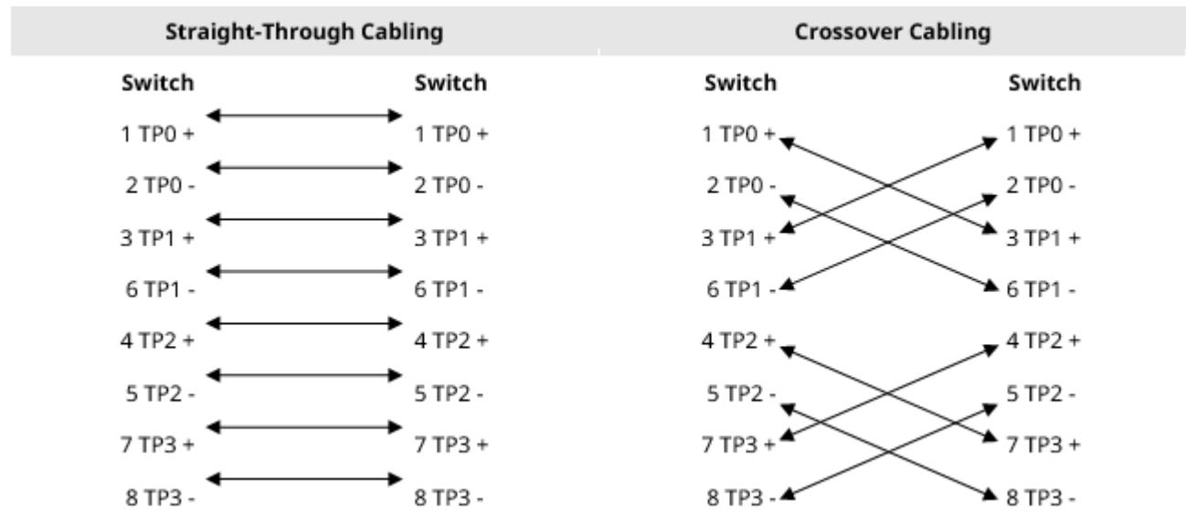
In addition to cables with the above-mentioned specifications, the 100BASE-TX/10BASE-T port can be connected using 100-ohm Category 3, 4, and 5 cables for 10 Mbps data transmission speed and using 100-ohm Category 5 cables for 100 Mbps data transmission speed with a maximum connection distance of 100 meters (328.08 ft.). The following table shows 100BASE-TX/10BASE-T pin assignments.
