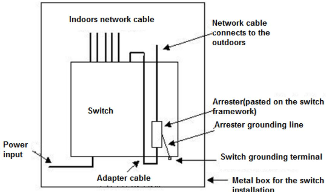
The Ethernet port arrester is only for the 10M/100M copper Ethernet ports with the RJ-45 connector;
