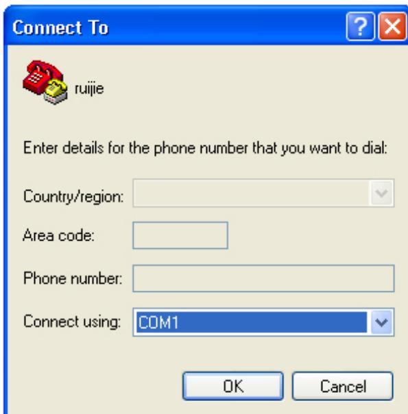
(4) After the serial port is selected, click **OK**. The Serial Port Parameter Setting window is displayed, as shown in [Figure 4-4](#). Set the baud rate as 9600, data bit as 8, parity check as none, stop bit as 1, and flow control as none.
