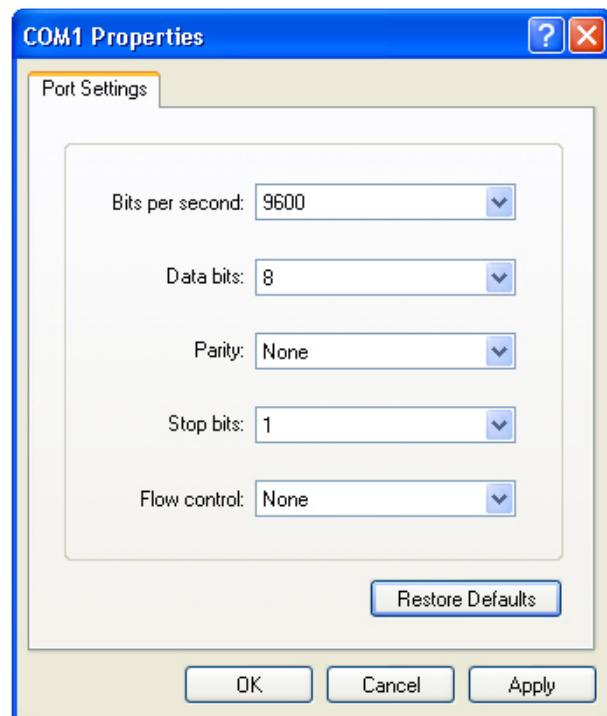
(5) After the serial port parameters are set, click **OK** to enter hyper terminal window.
