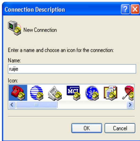
(3) Enter the name of the new connection and click **OK**. A window appears as shown in [Figure 4-3](#). In the column of Connect Using field, select the serial port you want to use.
