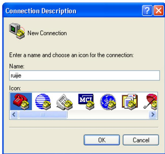
(3) In the Connectivity Note window, enter the name of the new connection and click **OK**. A window appears as shown in [Figure 4-3](#). In the Connect Using field, select the serial port you want to use.
