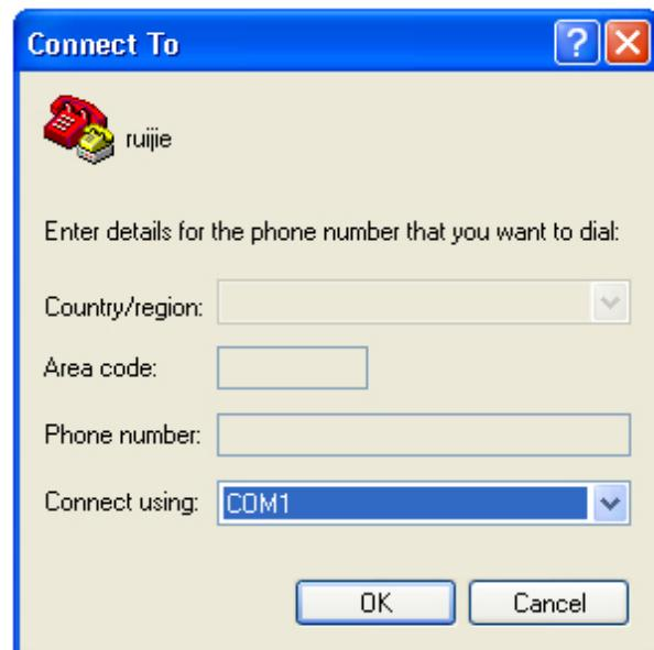
(4) After selecting the serial port, click **OK**. The Serial Port Parameter Setting window is displayed, as shown in [Figure 4-4](#). Set the baud rate to 9600, data bit to 8, parity check to none, stop bit to 1, and flow control to none.
