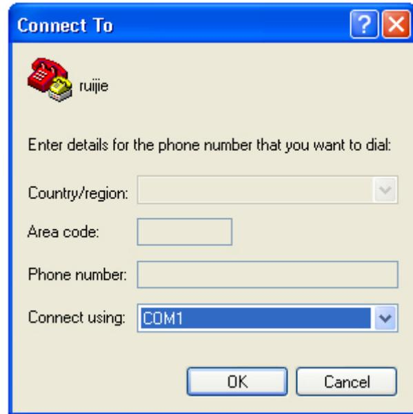
(4) Click **OK**. The **COM1 Properties** dialog box will appear. Select the following settings: Bits per second: 9600; Data bits: 8; Parity check: None; Stop bit: 1; Flow control: None.
