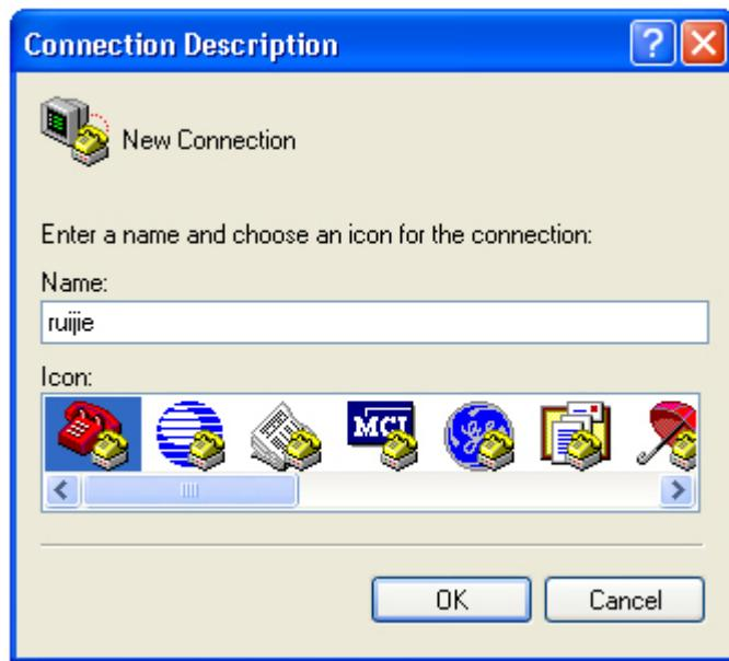
(3) In the **Name** box, enter the new connection name and click **OK**. The **Connect to** dialog will appear. From the **Connect using** drop-down list, select a COM port to be used.
