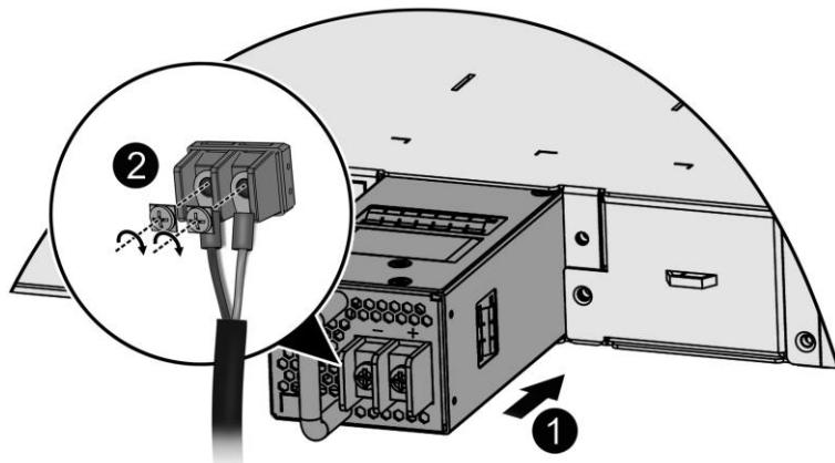
**Figure 3-8 DC Terminal Block**
