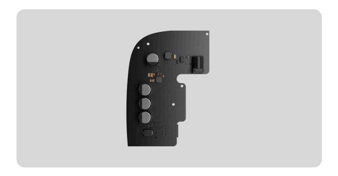
**12-24V PSU (type A)** is an alternative power supply unit to connect an Ajax hub or range extender to an 8–32 V= power supply. 12–24V PSU is an electronic board built into the control panel enclosure, replacing the standard 110/230 V~ power supply unit.
