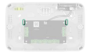
The device is fixed in two positions. You can turn it 180°.
