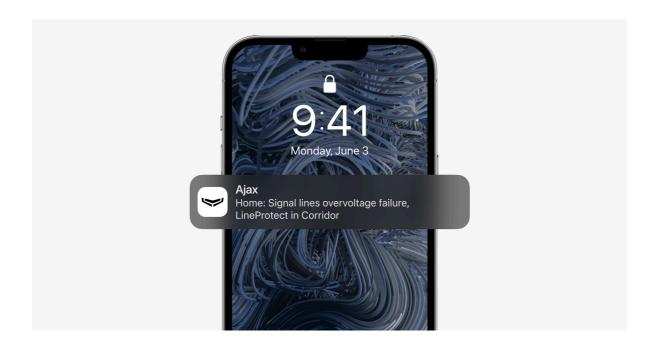
Fuses are triggered if an abnormal voltage is supplied on the Fibra line. In this case, LineProtect can fail, so it needs to be replaced. The users and the security company will receive the corresponding notification.
