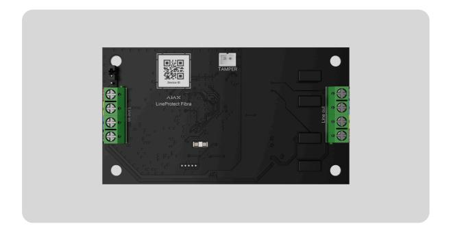
**Superior LineProtect Fibra** is a module designed to protect devices on the Fibra line from short circuit and sabotage: 110/230 V~ voltage supply to the line, hit with the stun gun.
