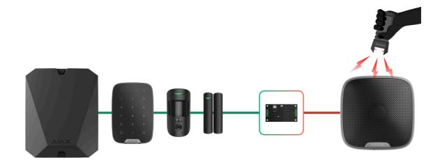
You need to connect one input and one output Fibra line to LineProtect.
