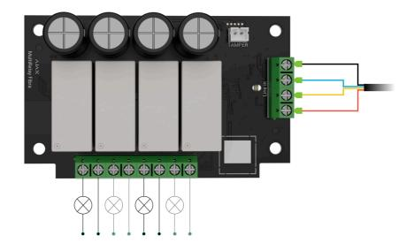
Each relay has potential-free (dry) contacts. Dry contacts are electrically isolated to the relay's power supply. Thus, this device can be used in low-voltage and household networks, for example, to simulate a button, or a toggle switch, or to control water shut-off valves, electromagnetic locks, irrigation systems, gates, barriers, and other systems.
